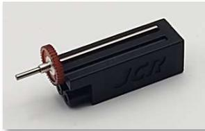
The jig also has two holes for inserting complete gear/axle sets and drilling holes to lighten the gears, using one of the various gear drilling jigs. Putting the axles in this jig for drilling, allows you to use a drill press, table, or hold it in your hand, without risking your fingers, and helping ensure you are drilling perpendicular to the gear.
